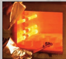
Headed blanks are heat-treated,
