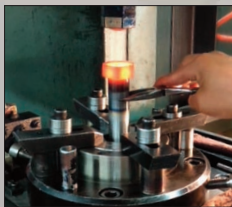
The red hot slug is brought to the press
