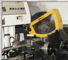
Bars are cut to length on our fully-automated bar saw.
