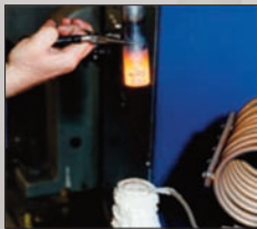
The red hot slug is brought to the press
