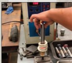
The trimmed slugs are induction heated.
