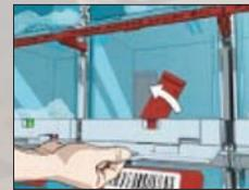
**4.** Pull the slider to drop stock from the top into the bottom bin. Flag raises to indicate the top bin requires restocking.
