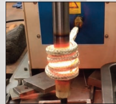
The trimmed slugs are induction heated.
