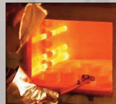
Headed blanks are heat-treated,
