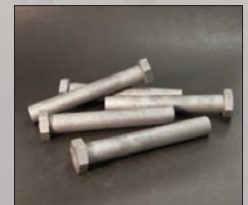
media blasted and descaled
